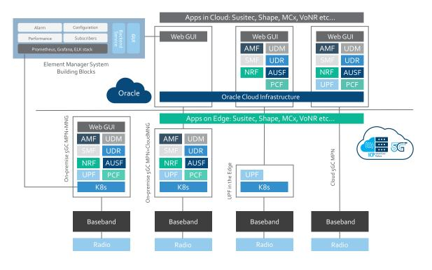
The 5G core runs on a security-optimised Ubuntu OS, where all network functions are virtualized with containers and orchestrated by Kubernetes. Optimal performance can be achieved by using Kontron's Intelligent Cloud Platform (ICP), but other platforms such as OpenStack, VMware and Oracle Cloud Infrastructure are also supported. The system is hardware and platform independent, enabling seamless integration into various cloud environments.
