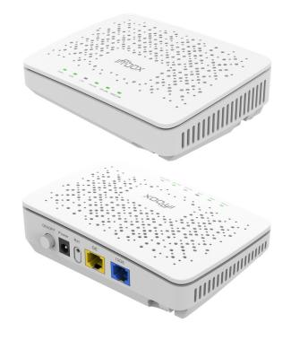
Iskratel Innbox X24 is a compact XGS-PON ONT that delivers advanced multi-gigabit services for an unparalleled user experience. Its XGS-PON WAN interface supports symmetrical data rates of 10 Gbps in downstream and upstream, while its multi-gigabit LAN interface supports 10 Gbps, 5 Gbps, 2.5 and 1 Gbps on the same port.
